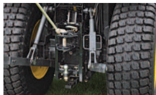
Height Adjustable Rear Hitch: Easy to use height adjustments for all trailers with clevis and ball type.
